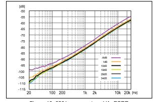
Figure 10. 6261 preamp stage VA- PSRR vs. frequency & gain.
