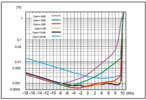
Figure 5. 6261 THD+N vs. output swing at different gains.
