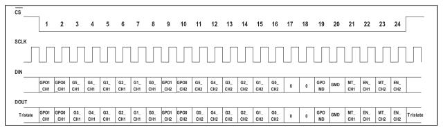
Figure 14. 626x 24-bit SPI control word definition.
