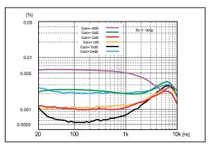
Figure 6. 6261 THD+N at Vout=1Vrms vs. frequency, 22kHz BW.
