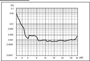
Figure 4. 6261 THD+N vs gain, f=1kHz, Vout=2Vrms
