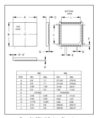
Figure 21. QFN-48 Package Dimensions
