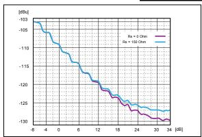
Figure 3. 6261 EIN vs. gain,  $0\Omega$  and 150 $\Omega$  termination.
