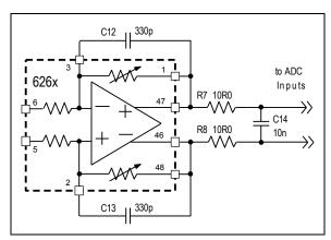
Figure 18. THAT 626x ADC driver in an alternate anti-aliasing filter configuration.
