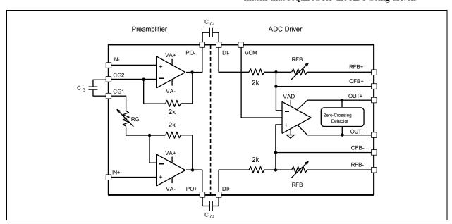
Figure 12. Analog Section Functional Block Diagram
