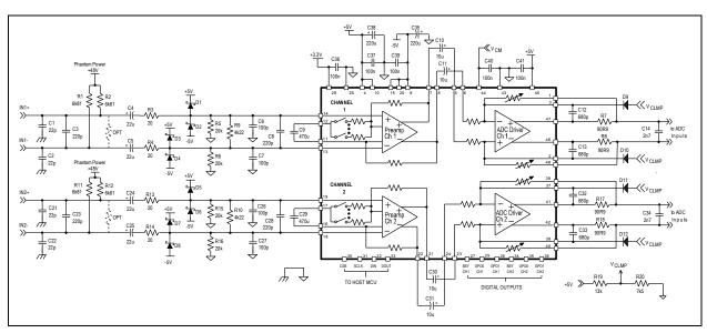
Figure 17. A typical bipolar-supply THAT 626x application circuit. See also Figure 18 for an alternative ADC anti-aliasing filter configuration.
