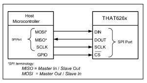
Figure 13. Single 626x connected to a host controller.
