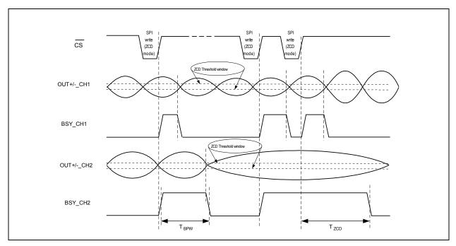
Figure 19. Timing diagram for the Zero-Crossing Detector and Busy Pin operation.
