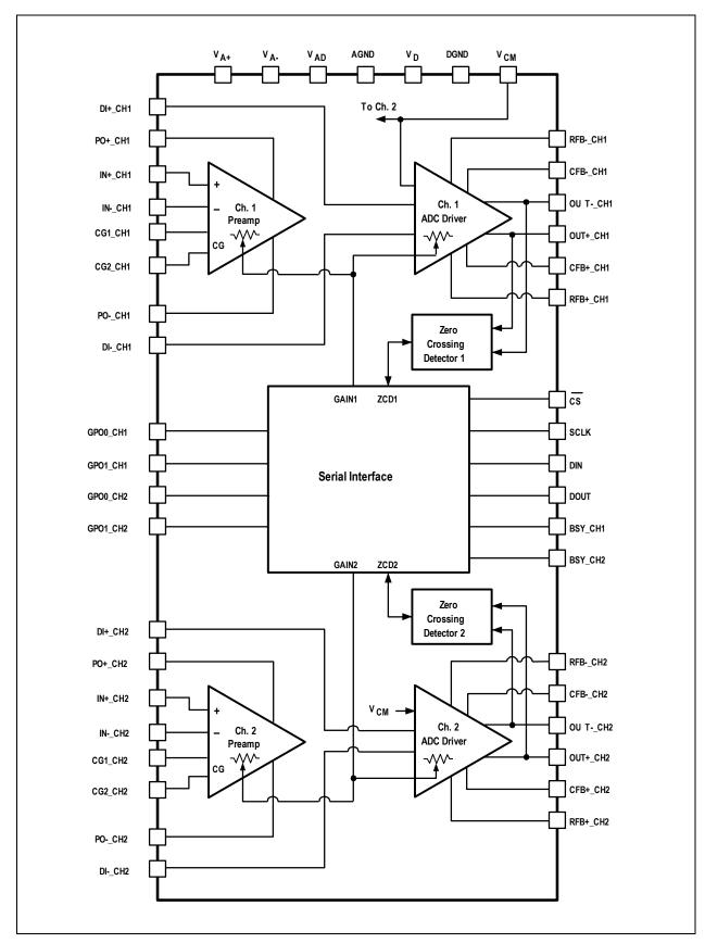
Figure 11. 626x block diagram.
