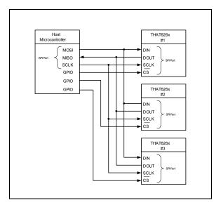
Figure 15. Multiple 626x ICs connected in parallel to a host microcontroller, with independent chip selects.
