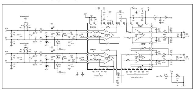
Figure 20. A typical unipolar-supply THAT626x application circuit. See also Figure 18 for an alternative ADC anti-aliasing filter configuration.
