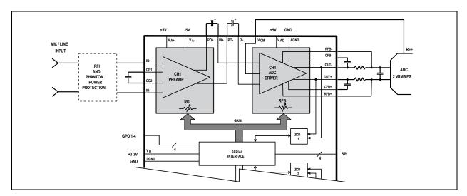
Figure 1. 626x simplified block diagram, bipolar supplies (one channel shown).
