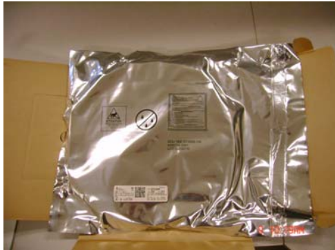
Figure 12 GD75232DWR devices in original sealed moisture barrier bag.
