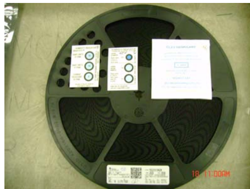
Figure 14 TSC2101IRGZR devices in original tape and reel with 1 desiccant and moisture indicator labels.
