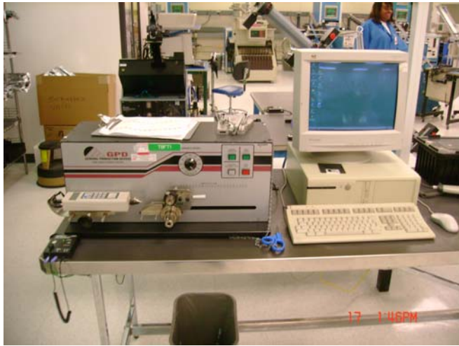
Figure 16 Peel-Back Force Test (PBFT) System.
