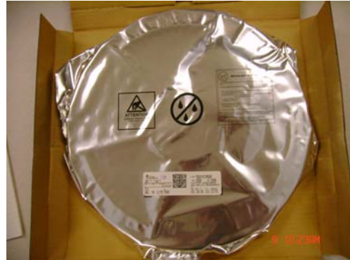
Figure 13 TSC2101IRGZR devices in original sealed moisture barrier bag.
