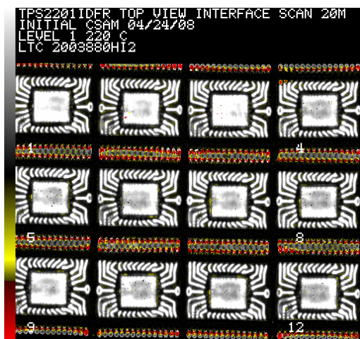
Figure 7 CSAM image of TPS2201 prior to moisture/reflow simulation. No significant delamination observed.
