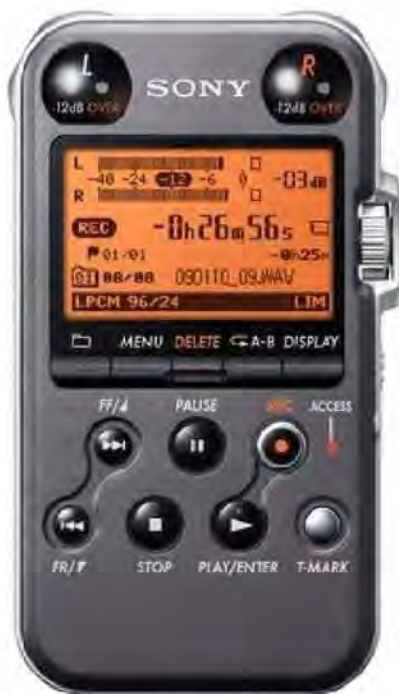
PHOTO 4: Sony's PCM-M10 palm-sized professional digital recorder, which records linear PCM at sample rates up to 96kHz with up to 24-bit resolution. The recorder has 4GB flash memory, and a pair of built-in omnidirectional microphones. (Courtesy of Sony Corp.)
