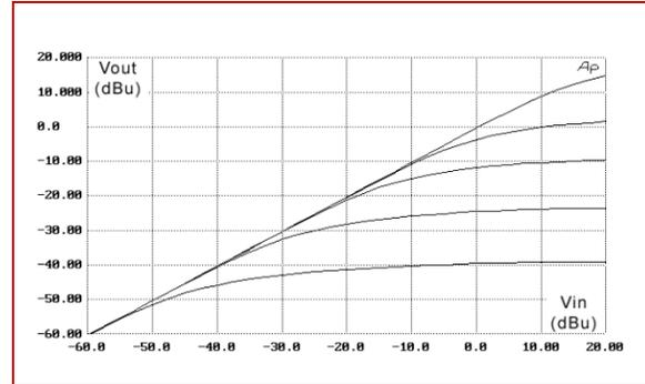
Figure 9.  $V_{OUT}$  vs.  $V_{IN}$  for the Soft-Knee Circuit.
