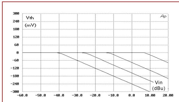
Figure 2. V<sub>TH</sub> vs. V<sub>IN</sub> for various THRESHOLD settings.
