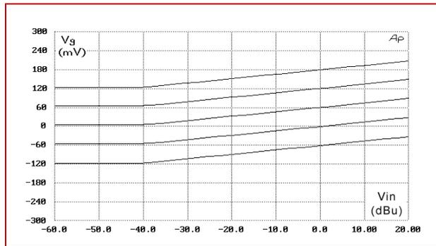
Figure 4.  $V_G$  vs.  $V_{IN}$  for various GAIN settings.
