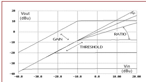
Figure 5.  $V_{IN}$  vs.  $V_{OUT}$  for various Control Settings.
