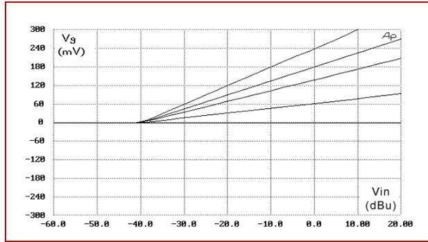
Figure 3.  $V_G$  vs.  $V_{IN}$  for various COMPRESSION settings.
