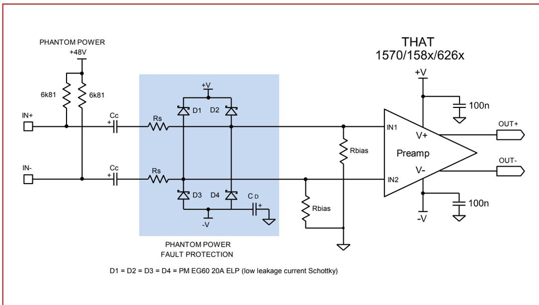
Figure 2. Phantom power fault protection scheme for THAT1570/158x/626x.
