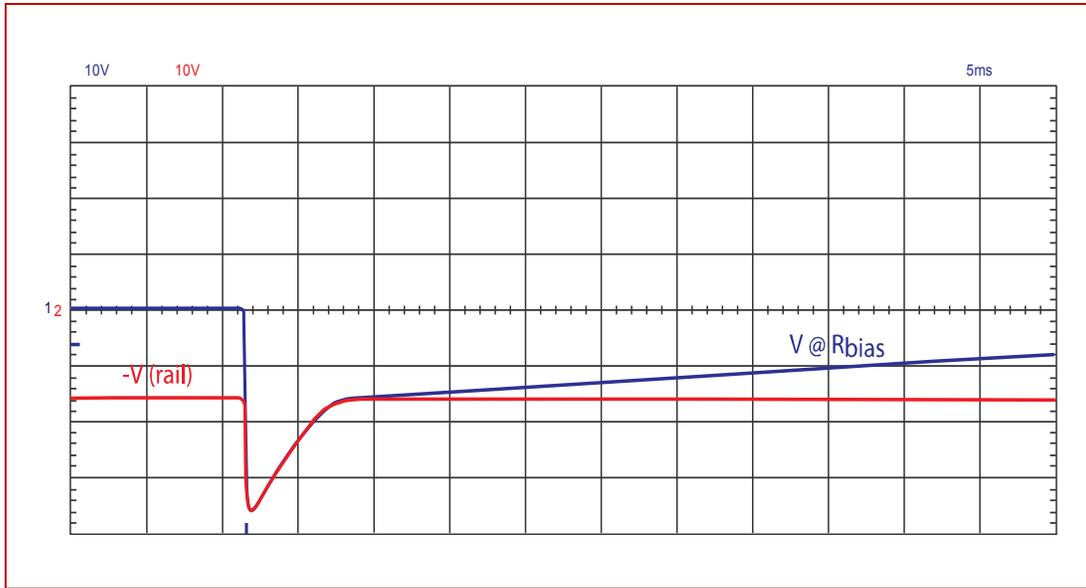
Figure 3. Impact on -V (red trace) during a phantom power fault [1] and [2].
