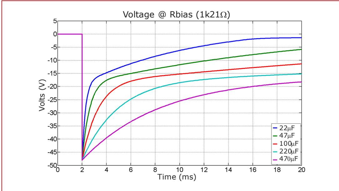
Figure 1. Voltage at Rbias during a phantom power fault for different values of  $C_c$  [1] and [2].
