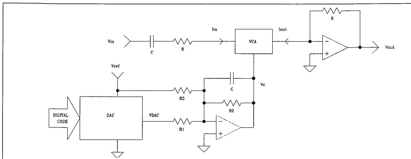
Figure 3 - VCA with Linear Control DAC
