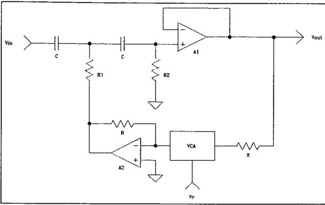
Figure 18 - Variable-Q Sallen and Key Highpass
