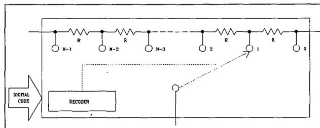
Figure 1 - Digitally Controlled "Pot"
