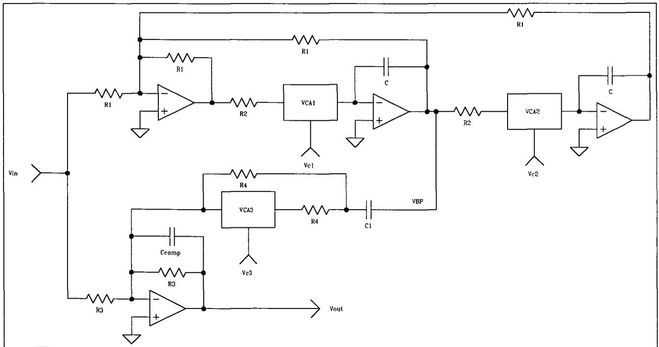
Figure 17 - Simplified VCA-Controlled Asymmetrical Parametric Equalizer
