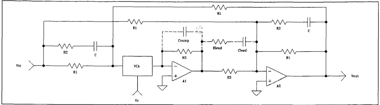
Figure 5 - VCA-Controlled High Frequency Shelving Filter
