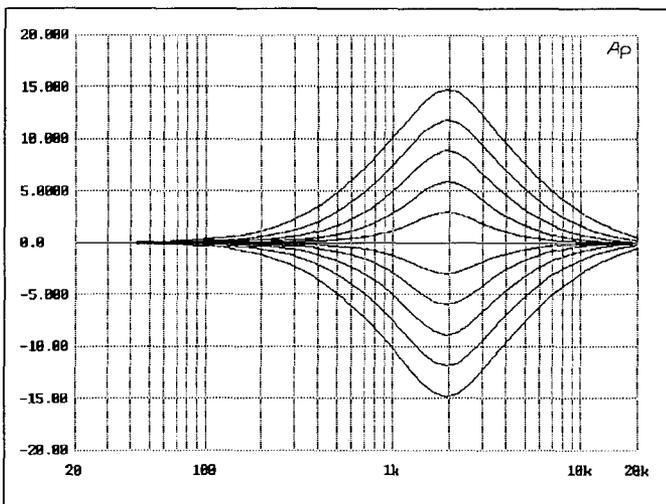
Figure 13 - Symmetrical Parametric EQ Responses for Boost and Cut (G<sub>3</sub> varied in 3 dB steps)
