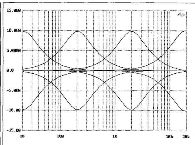
Figure 14 - Symmetrical Parametric EQ Responses (V<sub>freq</sub> varied in "20 dB" steps)
